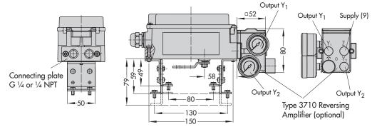
Mounting unit CrNiMo steel bracket
